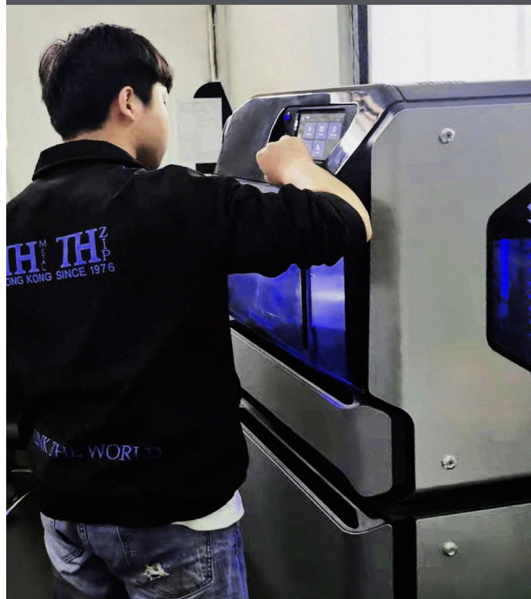
TH Zipper uses the Stratasys J55 to make pullers and buttons prototypes
