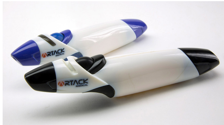
This articulated hernia mesh fixation device prototype was 3D printed complete with logo.
