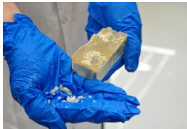
Figure 5 and 6: Peeling the support material from the printed model.
