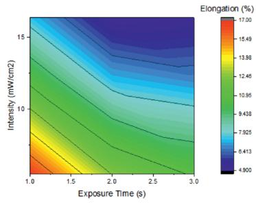
Printing parameters influence the degree of conversion and ultimately on part performance, in this case how modifying UV exposure intensity and time affects percent elongation.
