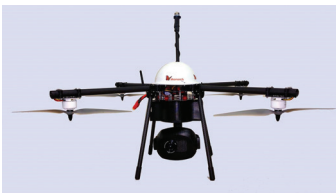
A 3D printed cocoon housing hangs between the legs of Monarch agricultural drone.
