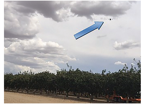
This special Monarch drone plays audio recordings of predators to scare away birds from crops.
