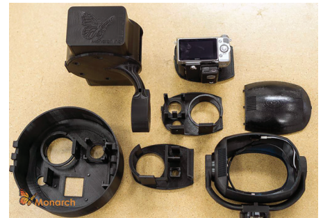
A sample of 3D printed parts (not including the camera shown at top) that make up a Monarch drone.
