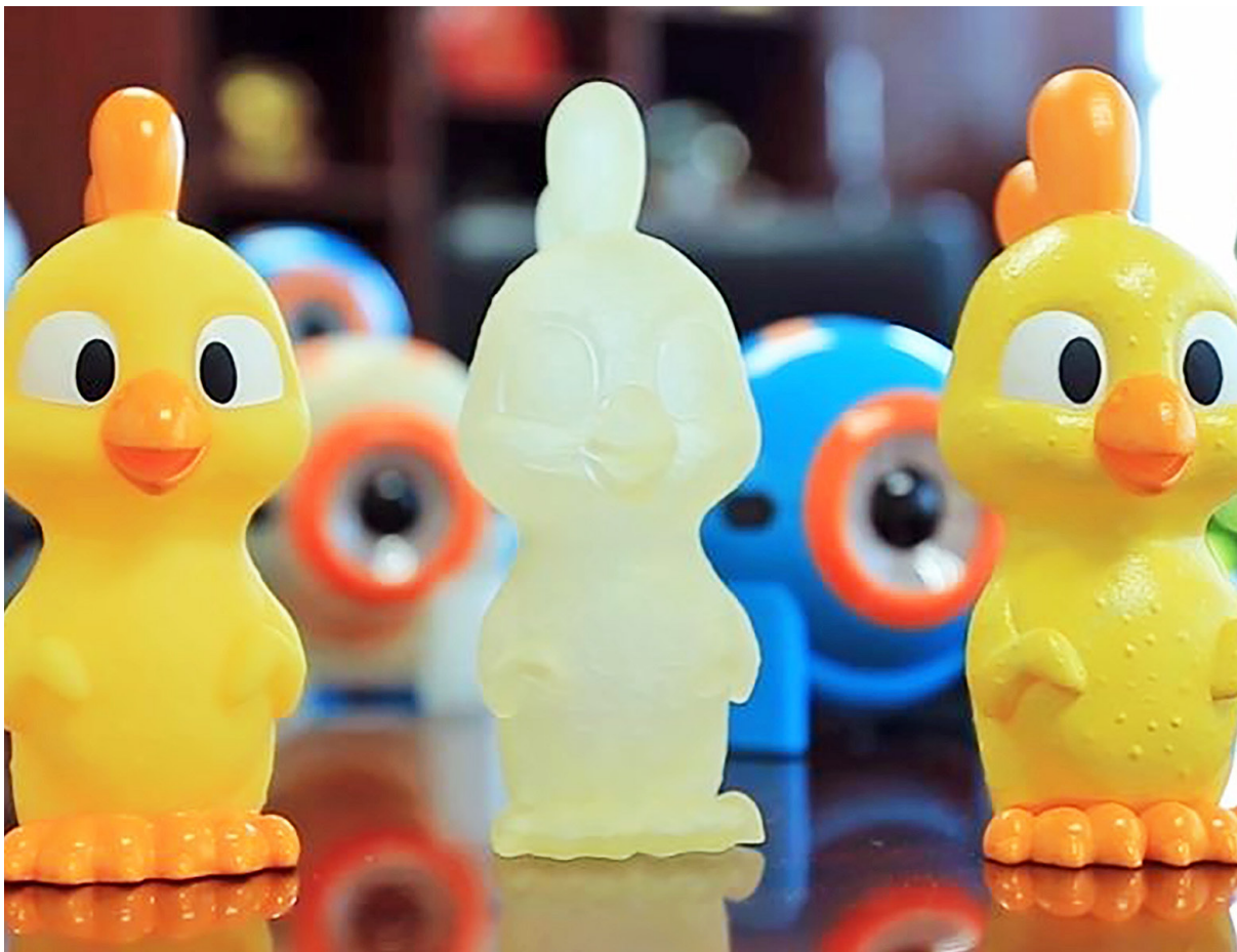
3D printed models (middle and right) shown with the final mass-produced product (left).
