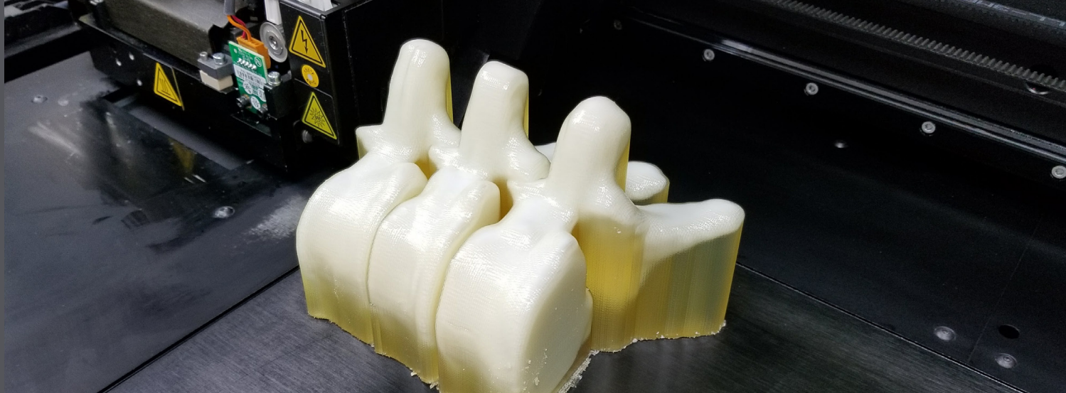
Vertebrae models used for medical device testing, printed on a Stratasys PolyJet 3D Printer.
