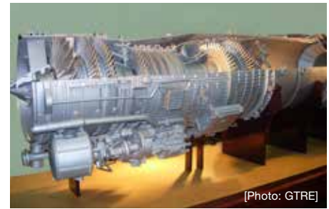
The Kaveri engine prototype had 2,500 FDM parts. [Photo: GTRE]
