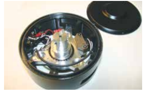
The FDM enclosures are loaded with electrical, mechanical, and optical components.
