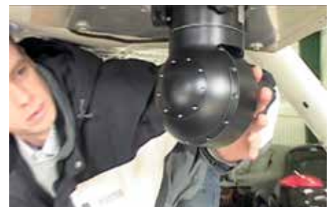
The COLIBRI is mounted on a helicopter and tested.
