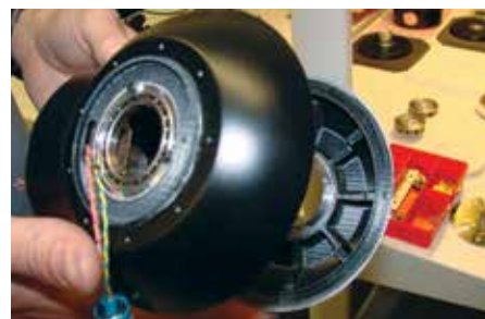
Direct digital manufacturing: FDM is used to produce 20 of the COLIBRI's components, including the enclosure.
