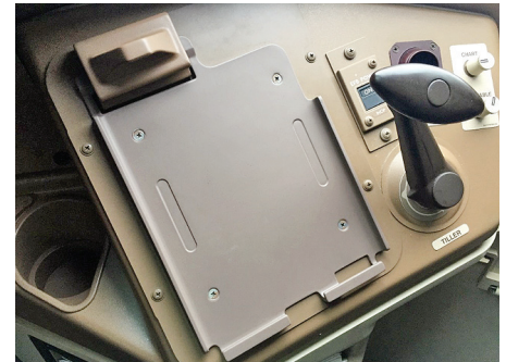
The 3D printed electronic flight bag support device installed by Eastern Airlines Technic AM lab.
