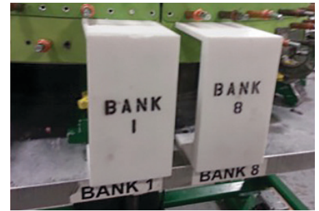
3D printed templates inspect contoured panel edges
